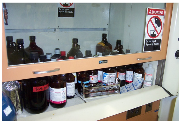
Figure 12: Improper Fume Hood Storage
